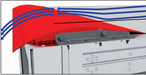
The Aero Rain Guard compresses and redirects high energy airflow on the trailer roof around the rear corner and down into the low energy trailer wake.
