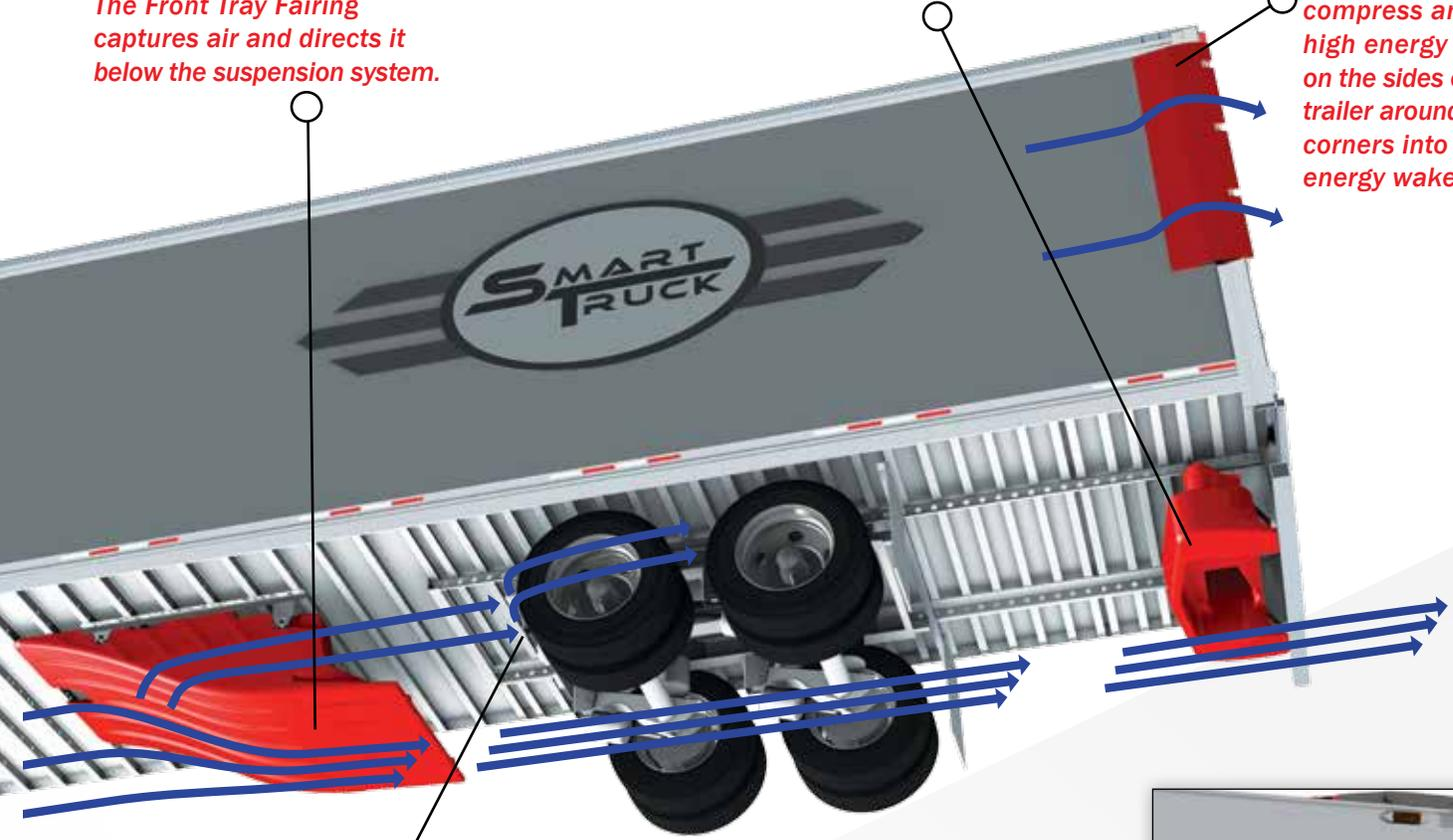
Increased airflow coming from the side of the Front Tray helps tire and brake cooling
